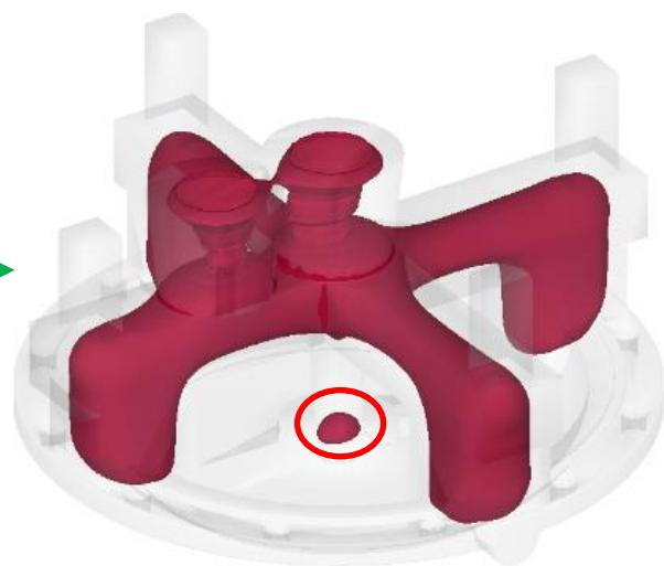
Liquid fraction analysis shows isolation at the center boss portion. At the same location, shrinkage porosity is also seen.
