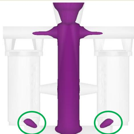
Solidification temperature analysis shows isolated temperature region at bottom side, which leads to shrinkage at the same location of shop floor defect.
