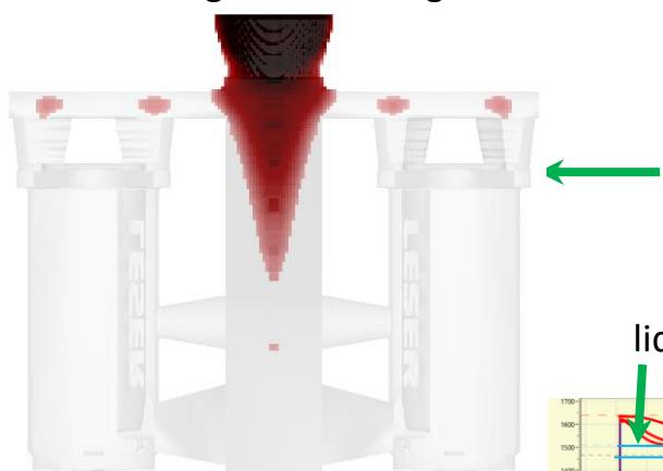
Thermocouple analysis reveals that thermocouple in part region crosses solidus temperature earlier and thermocouple at sprue crosses solidus afterwards thus sprue solidifies last.
