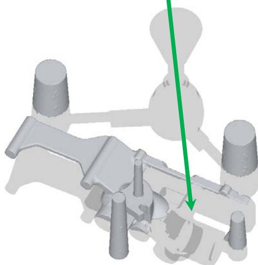
**Summary:** The revised methoding with flow-off was used to solve the blow hole defect. Simulation helped in saved large shop floor time and allowed user to analyze large no. of methodings to solve the defect
