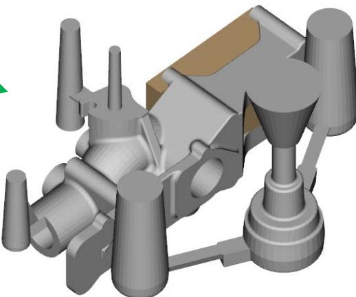
Simulation results indicate good casting with no isolated air pockets. Changes in methoding were able to solve the blow hole defect.
