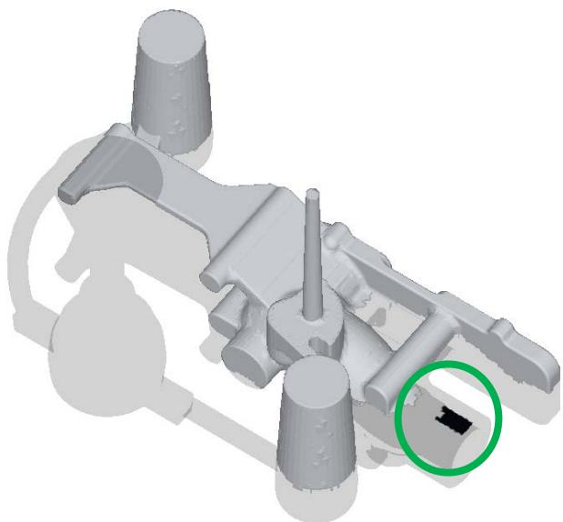
Simulation was done to understand the effect of new methoding. Air porosity analysis indicates presence isolated air pockets. These locations match with the isolations seen with the earlier methoding. The results suggest more changes have to be done in methoding to remove the defect.
