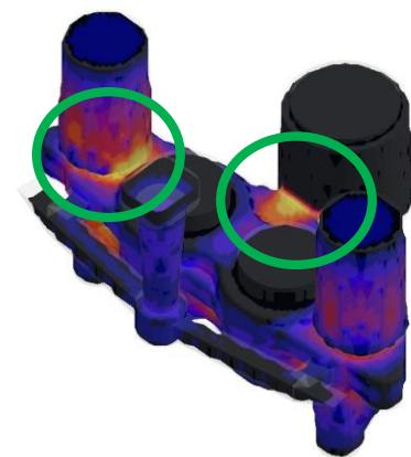
Shrinkage porosity is observed in the feeders. Shrinkage porosity from casting is completely eliminated.
