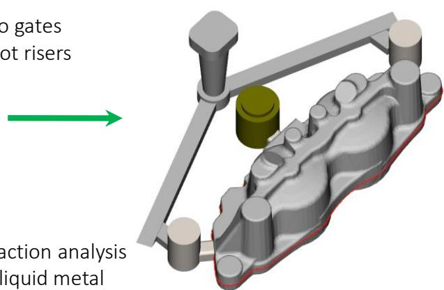
Liquid fraction analysis displays liquid metal remains inside the casting till the end of solidification. These locations can lead to shrinkage porosity.
