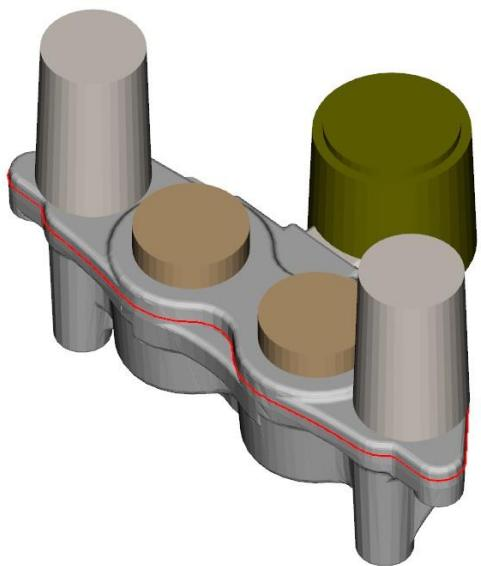
The solidification map of revised methoding indicates uniform and directional solidification with entire hotspot region shifted to the feeders
