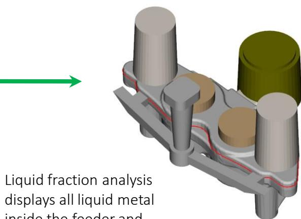
Liquid fraction analysis displays all liquid metal inside the feeder and sprue at the end of casting.
