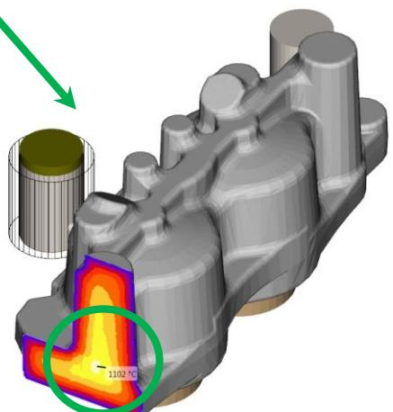
Solidification and feed path simulation reveal isolated hotspot around the side boss section, exactly matching the defect found in the casting.
