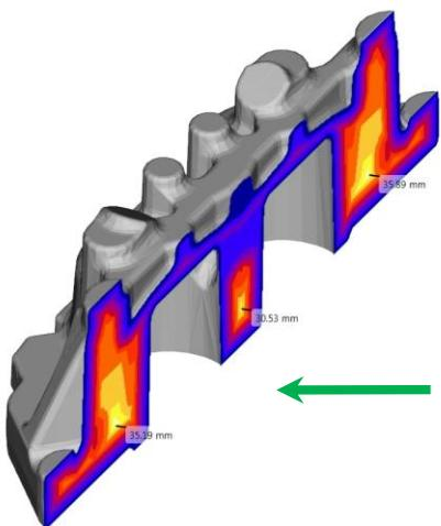
Thickness analysis of the part shows varying values with a maximum of 35 mm at the side boss and 25 mm at the central boss, connected by a thick section.
