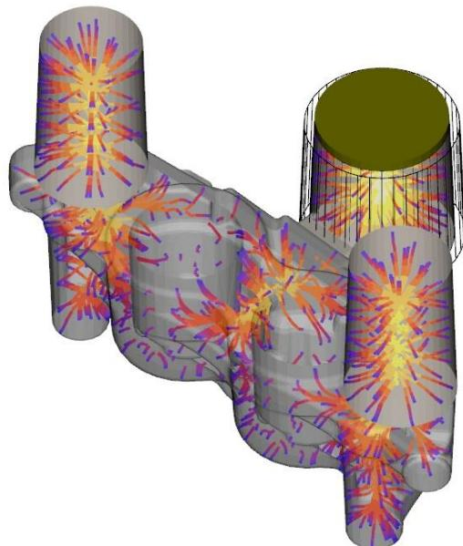
A closer investigation of the critical sectional view and the feed path analysis shows the favorable temperature contour and the feed paths well connected towards the feeder.
