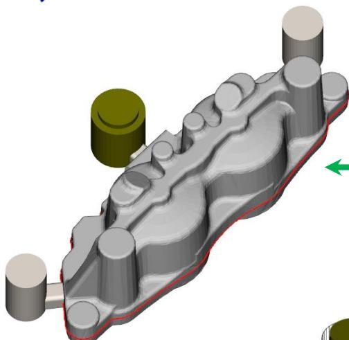
Initial method of the casting included three side feeders, all connected close to the thickest section to address the hot spots. An insulated sleeve is also provided to the central feeder to increase its effectiveness.
