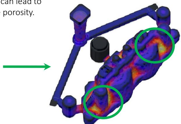
Shrinkage porosity is seen inside the bosses and matches with the defect seen in the part. The lighter colour shows micro shrinkages and darker colour shows macro shrinkages.
