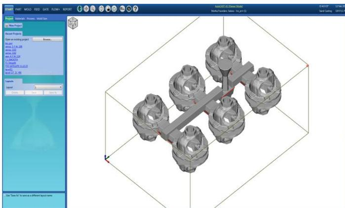
Fig.4.1. Modified gating with mold box
