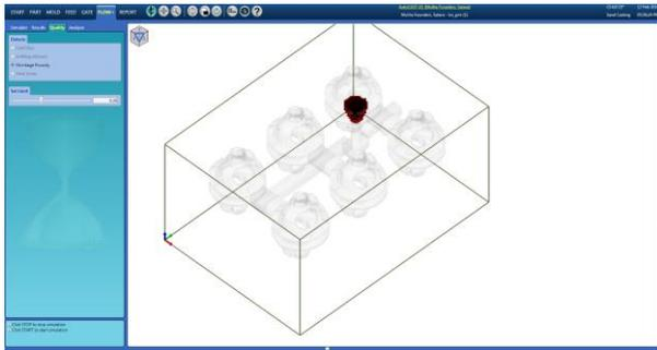
Fig.4.4. Modified design with no shrinkage porosity
