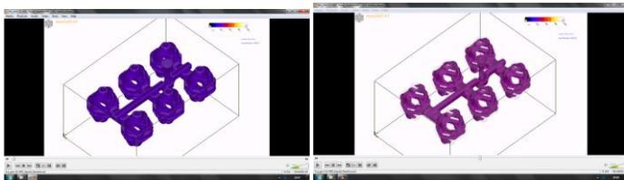
Fig.(a)97.87% of Liquid Fraction Fig(b).50% of Liquid fraction
