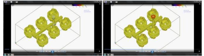
Fig.(a) 5% of Solidification Fig.(b) 50% of Solidification
