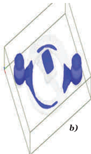
Fig.5 Solidification for gating ratio of 1:2:2, with a) temperature distribution and b) liquid fraction.
