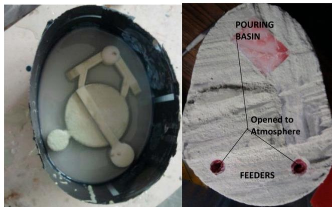
Figure 7. Mould Preparation
