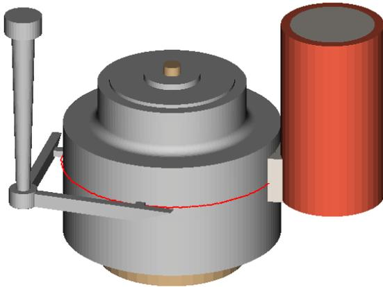
The revised methods design includes a larger feeder of height 200 and diameter 90 mm, also neck size is increased up to 50 X 50 mm dimensions.
