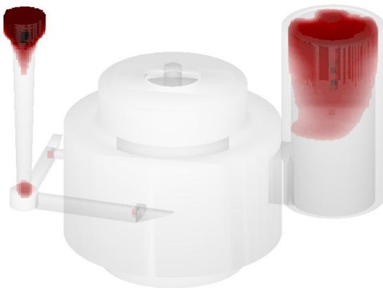
Shrinkage porosity results also shows that it is observed in the feeders only. Shrinkage porosity from casting is completely eliminated.
