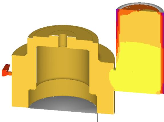
Solidification temperature analysis shows isolated temperature region inside the feeder. So casting is free from shrinkage defect.
