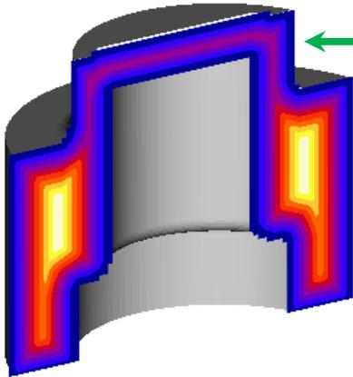
Thickness contour analysis of the part shows a thick region all around the part, equivalent to an inscribed sphere diameter of 60 mm.
