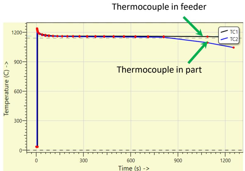
**Summary:** Simulation reveals that the modulus of neck is comparatively smaller than the feeder and casting section, thereby altering the dimensions of feeder and feeder neck, resulted in defect free casting.
