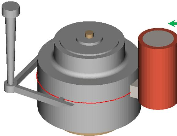
The current methoding of the casting included a cylindrical side feeder of 70 mm diameter and 160 mm height with a insulating sleeve of 10 mm. The dimensions of square neck used are 30 X 30 mm.
