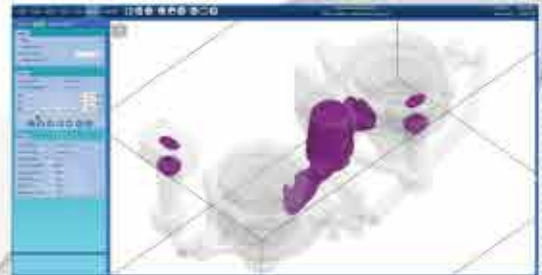
Liquid fraction of solidifying metal
