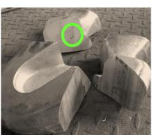
Simulation of current methoding indicates an isolated hot spot just below the feeder connection. This exactly matches the shrinkage defect found in the actual casting.
